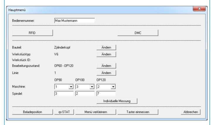
The customer-specific user interface means that your special requirements can be easily catered for. The measuring machine does not, therefore, need to be operated by trained measuring staff. The respective measuring program sequence can be selected automatically by reader using the RFID and data matrix code on the workpieces. This prevents allocation errors by the user.
